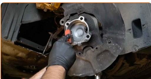
**36** Install the new wheel hub with a bearing.
