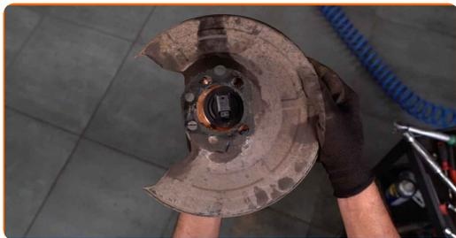
**33** Install the new wheel hub with a bearing.
